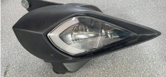
5.Install the new light in the same way as the removing of the original light, and fix it with the spare screws removed before (connect the plug-in of wiring harness on the light with the plug-in of wiring harness on the vehicle before installing the headlight), for the other side, replace the headlight as above Steps 2-4. As shown in figure:
