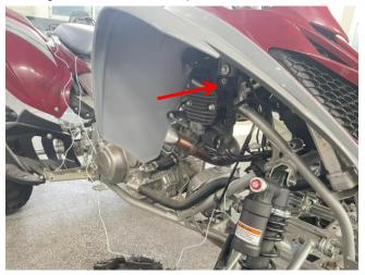
3. There are three O-shaped rubber rings and a stainless steel round tube on the removed original lamp, install the O-shaped rubber rings on the new headlight as the position of the original headlight, and
