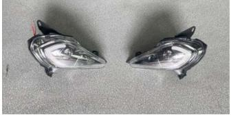
2. There is a fixing screw for the original headlight, unscrew it for later use. Remove the original headlight, as shown in the picture:
