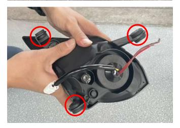
4. Install the outer decorative frame of the headlight, find the corresponding position, and directly lock it, as shown in the picture:
