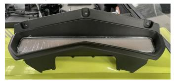
2. Remove the cover of the original vehicle, remove the decorative panel on the cover, install the hood accent light, and fix it with screws. As shown in picture:
