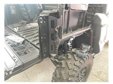
2. Install a new taillight, fix it with the original vehicle screws, and then reconnect the overall harness with the taillight wiring harness. Then start the vehicle first, check whether the taillight works normally, and finally install the leaf plate back to its original position (the other taillight can be replaced and installed according to the above steps). As shown below:
