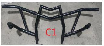
3. Assemble part C1 and part D with four M8\*16 inner hexagon screws.
