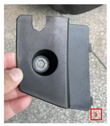
3. Fix the license plate lamp on the bracket, tighten the screws, and fix the wire harness with tie tape according to the position of the wire groove.
