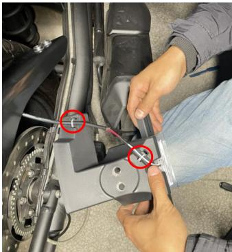
4. Install the license plate lamp and bracket into the fender in the correct direction, and the screw fixing position on the back of the fender is reinforced with nuts.
