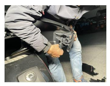
5. Remove the 2 screws that fix the heat shield on one side of the vehicle, remove the heat shield, and unplug the harness plug of the original vehicle.
