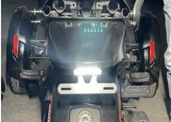
7. Install the fender on the vehicle, install the removed plug cover (the plug cover with notch is installed on the right), fix the screw from below the fender, and install the license plate lamp.
