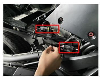
6. Use the wire harness on the license plate lamp to pass through the wire hole on the
