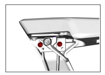
5. Install the assembled armrest using [P6] Torx truss screw M8 X 30 screws and plate [P5].
