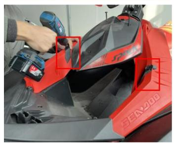
5. There are two bayonets in the middle of the lower frame of the storage box. Press the top of the storage box lid against the bayonet, then the lid can be installed, as shown in the
