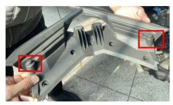
3. Then fix the the lower frame on the front cover device of motorboat, hold it by hand, follow the screw hole positions on the frame, drill holes by 4.5mm drill bit, and then fix with screws. As shown in picture:
