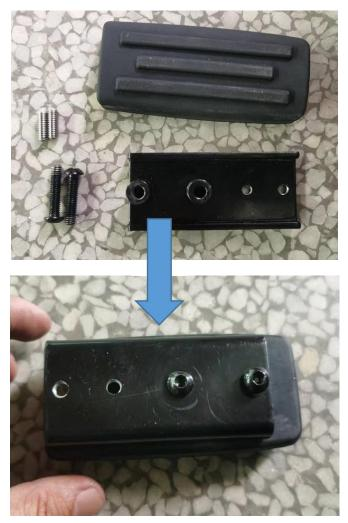
3. Fix the pedal on the iron bracket with two screw rods, do not tighten, and insert the pedal into the pedal frame, as shown in the figure.
