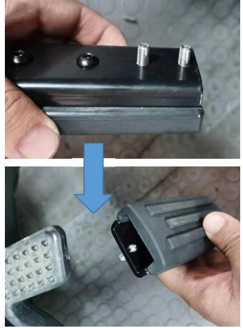
4. Tighten the screw to fix the iron bracket, and the installation is complete, as shown in the figure.
