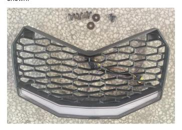
2. Remove the bumper and mesh grille of the original vehicle, and remove the three steel clips on the back of the original mesh grille for standby.
