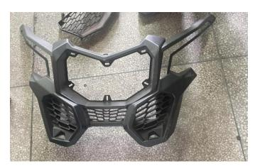
3. Install the three steel clips of the original mesh grille on the new mesh grille, then install the new mesh grille back on the bumper and fix it with two screws.
