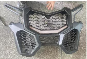
4. Install the bumper back into the vehicle, and then connect one end of the harness plug-in of the new mesh grille to the original vehicle harness plug-in, and the other end to the position lamp harness plug-in.
