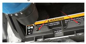
5. Hold in place and counter-drill with a 4mm drill bit. Use 6.5x30 self-tapping screws to fix the device holder on the dashboard.
