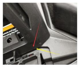
4. Hold in place and counter-drill with a 6.5mm drill bit. Use M6X20, M6 flat washer, and lock nut to fix the device holder on the dashboard. NOTE: Do not tighten the screws now.
