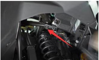
3. Remove the front bar, remove the front net and the net lamp (the screws on both sides of the net need to be removed).
