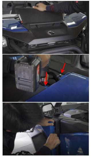
2. Remove the 8 screws that secure the front bar.
