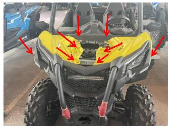
2.Remove the 10 screws that secure the front bar, and remove the front bar.
