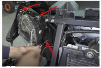
5. Install the screw rod from the original light and the rubber pad from the mounting hole onto the LED headlight.
