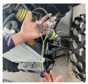
6.Install the LED headlight back to the original position and fix it according to the previous removal method (Note: the stainless steel flat pad and rubber ring of the original light must be used when fixing the screw). After that, install the front bar, covers and decorative plates on both sides.
