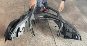
4. Remove the original lights protective shell from the back of the removed bumper, remove the light and replace it with the LED headlight (install the other side according to the same steps).
