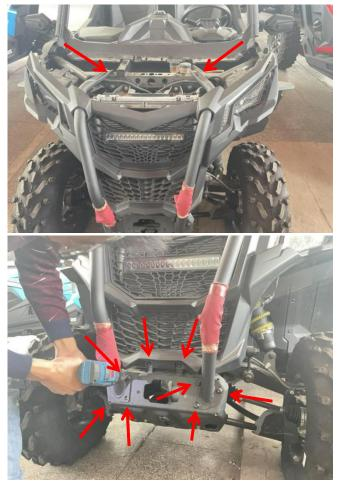
3. Remove wiring harness plugins from the original headlights and remove the entire bumper.
