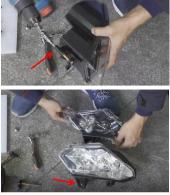
6. Install the LED headlight back to the headlight bracket in the way previously removed, and connect the corresponding wiring harness plug-in (install the other side according to the same steps).
