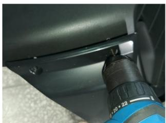
5. Use screws to install air intakes on both sides of the net.
