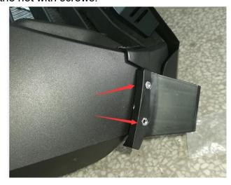
4. Clamp the narrow section of the air inlet onto the mounting bracket, and attach the wide end to the upper part of the middle net on both
