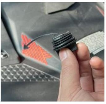
3. The drain plug arrow is upward, insert it into the plug and rotate it for several turns (install the other side in the same way).
