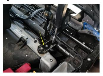
4. Install the llight bracket assembled in step 2
