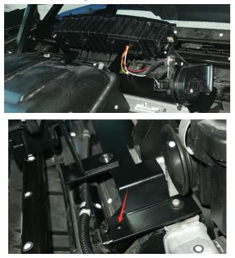
5. Take power from the original headlight harness through the adapter cable. **Note:** For models 2019 and up, it is only necessary to plug the conversion wire of the headlight with the headlight wire of the original vehicle, and replace the decorative cover in front of the headlight with the decorative cover in the accessory bag.
