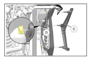
4. Install front LH light 1 to fascia using three retained nuts 0.
