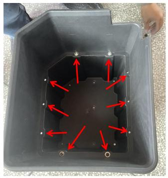
2. Lift the passenger seat, unscrew the 3-hole screws fixing the floor mat under the seat, and then place the assembled storage box in the installation position. Mark four fixed points with a marker according to the screw holes at the bottom of the storage box, then remove the storage box and drill the screw holes with a 3mm drill. As shown in figure:
