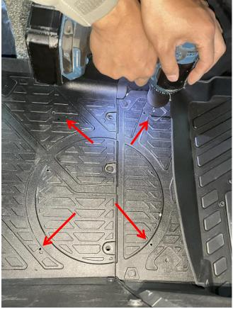
3. After above steps are completed, put the storage box back to the installation position, screw the floor mat screws that were
