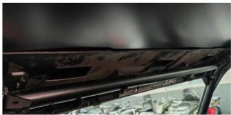
6. Attach the tail of the aluminum roof to the frame with two M6\*30 screws, M6 flat washers, rubber gaskets and two iron brackets, as shown in the picture.
