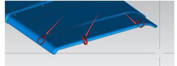
3. Align the 2 half roofs, fix them together by using M6x25 self tapped screws, forming a complete roof.
