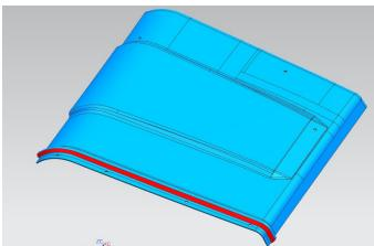
4. Secure the roof panel to ROPS by using M6X30 screws and 46mm hoops.
