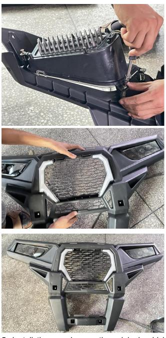
5. Install the new bar on the original vehicle and fix it with screws. Finally install the cover back . As shown in figure:
