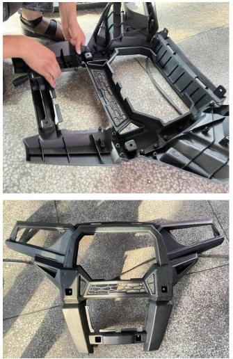
4. Remove the cover and front bar of the original vehicle and remove the headlights, mesh grill and rear brackets on the original bar and install them to the new bar in the original way. As shown in figure:
