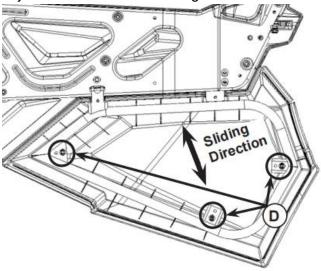
6. After adjustment, tighten the upper screws (10) to torque 16 ft. lbs. (21.7 Nm) and lower three screws to 5 ft. lbs. (6.78 Nm).
