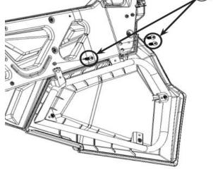
3. Install the screws (10) at three specific locations.
