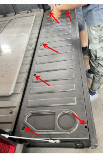
4. Remove the outer door panel, and remove the limit rods on both sides of the door panel and the door switch. Then replace the new switch with the original screws, and finally put the limit rods back in place. As shown below:
