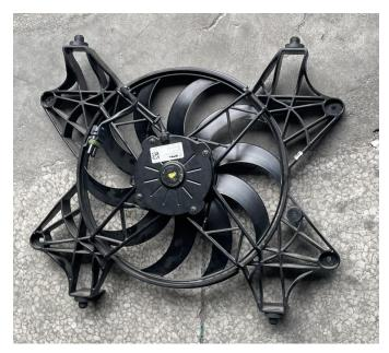
6. Install the assembled new fan bracket back on the vehicle, fix it with the original vehicle screws, and then reconnect the fan wiring harness with the vehicle wiring harness plug-in. As shown below:
