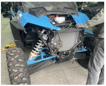
4. Disconnect the wiring harness plug-in of the fan of the original vehicle, unscrew the fan bracket of the original vehicle, and remove the fan bracket. As shown below:
