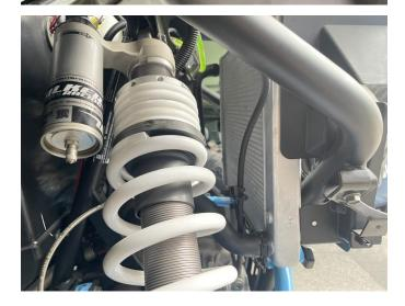
5. Remove the fan and other accessories from the original bracket and assemble them on the new bracket in the same position. Use nylon cable ties to secure the cable harness of the
