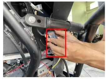
**5.** Connect the remaining wire harness of the #2 conversion cable to the wire harness of the rear accent light (stuck the plug-in of the connector in the rear shell of the rear accent light to prevent the plug-in from flooding when it rains), and then fix the rear accent light on the original vehicle with screws. As shown in figure:
