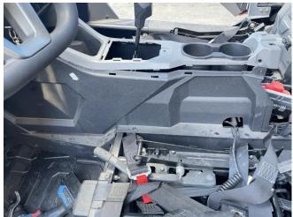
2. Open the cover of the center console storage box and take out the built-in tray. Prepare the 3M extension cable in the product, thread it through the center console and shift rod from the storage box, and then thread it through the outlet hole at the end of the armrest box to the rear wheel of the original vehicle. As shown in figure:
