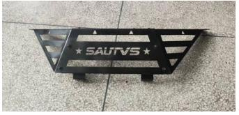
4. Remove the four screws on the rear frame of vehicle and set them aside. Install the rear tailgate in the position shown in the figure, and fix the tailgate firmly with the removed screws of the rear frame. The installation is complete.
