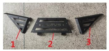
3. Assemble part 1, part 2 and part 3 with 6 hexagon screws of M6\*20, 6 lock nuts and 6 flat washers, as shown below:
