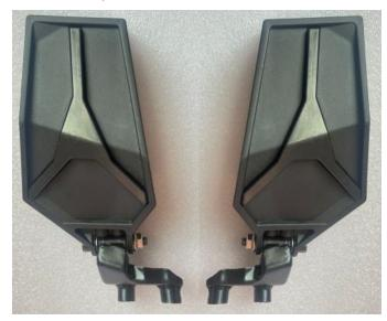
3. First remove the screws of pillar A of the original vehicle, install the side mirror on pillar A and then fix it with the screws in the accessories package, and install the other side in the same way. As shown below:
