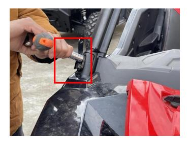
4. Install the side mirror on the bracket, fix it with the matching screws, adjust the Angle of the side mirror, and then tighten the screws (the side mirror on the other side can be installed in the same way as above). As shown below:
