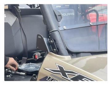
4. Install the side mirror on the bracket, fix it with the matching screws, adjust the Angle of the side mirror, and then tighten the screws (the side mirror on the other side can be installed in the same way as above). As shown below:
