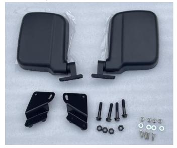
3. First remove the screws of pillar A of the original vehicle (hold the nut at the back with your hand to prevent it from falling out), fix the mounting bracket of the side mirror on pillar A with the matching screws in the package. As shown below:
