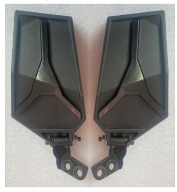
3. First remove the screws of pillar A of the original vehicle (hold the nut at the back with your hand to prevent it from falling out), install the side mirror on pillar A and then fix it with the screws in the accessories package, and install the other side in the same way. As shown below:
