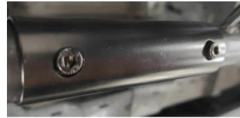
2. Fix the Spare Tire Carrier on the rear frame with eight M8\*35 inner hexagon screws.
