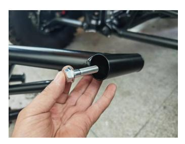
2. Install the lower end of the bumper at the position (shown in the picture) by two M10\*75 nuts with washer and two iron brackets.
