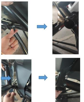
2. Fix the screws and install 2 plastic plugs.
