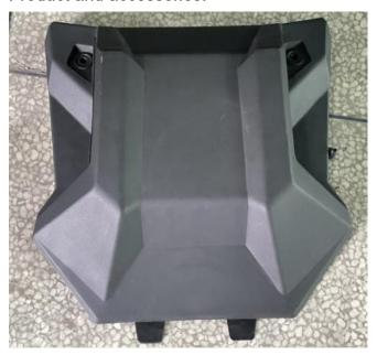
1. Remove the air inlet hood of the original vehicle, reinstall the new air inlet hood, and fix it with the expansion screws of the original vehicle. As shown in figure:
