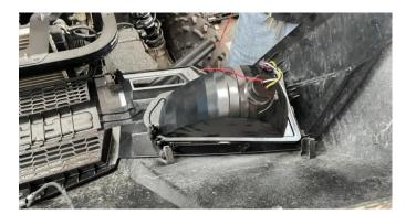
4.After installing the headlight, take out the transfer wiring in the accessories package, and connect one end with the headlight wiring harness. The other end is connected with the original wiring harness on the vehicle, as shown in the figure;
