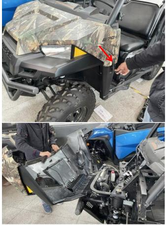
2.Firstly, remove the wiring harness plug-ins of the original headlight and remove the headlight (there is a steel clip and two O shaped rings on the headlight, remove them for later use) as shown in the figure:
