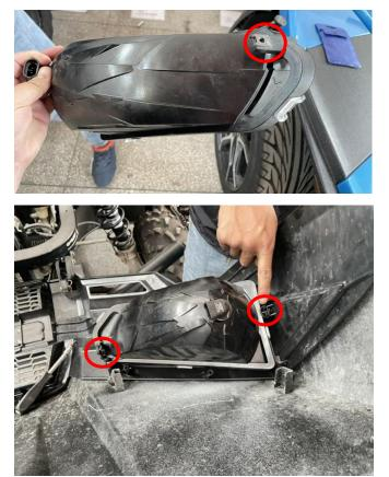
3.Place the removed steel clip to the new headlight following the position of the original headlight, and then install the light to the vehicle, and fix the screws, and the O-rings are also installed back to the original position, as shown in the picture:
