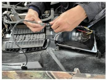
5.After connecting the headlight wiring harness, take out the white wiring that you prepare in advance, peel off the outer skin of one end, expose the copper wire, and connect it to the ACC
