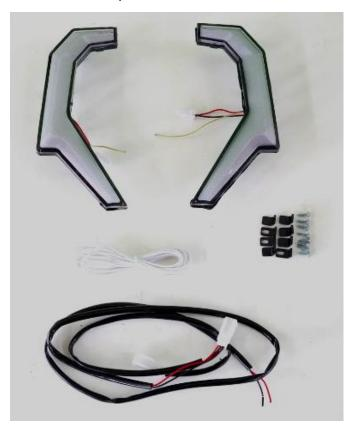
2. Remove the front mesh grill of the original vehicle, fix the lights on both sides of mesh grill with the little "L" brackets and screws in the product package. As shown in the picture:
