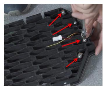
3. Remove the cover of the original vehicle, connect one end of the patch cord (in the package) to the terminal post of original vehicle, pull the other end to the central mesh grill, and connect with the accent lights wiring harness respectively, then install back the central mesh grill. As shown in picture:
