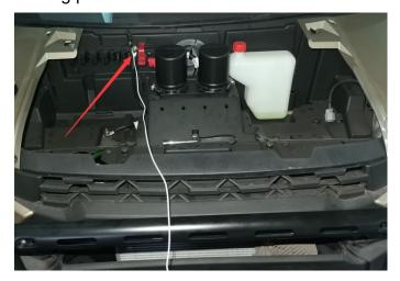
7. Connect the wire coming from ACC (positive) and the wire coming from the binding post (negative) to the plug on the mesh grill.
