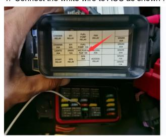
5. Wires go through the position as shown in Step 3.
