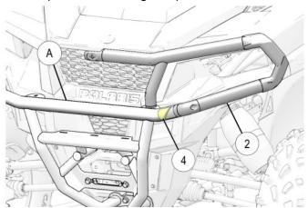
9. Loosely install screw 6 up through mounting ears in existing bumper A, then into LH bumper 2.
