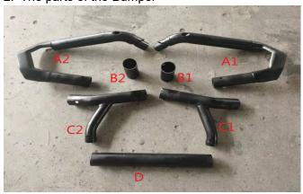
3. Assemble part A1, part B1, part C1 according to the diagram.
