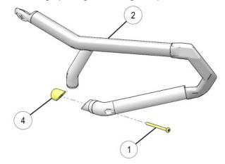
8. Fully insert threaded mount 4 and tapered end of LH bumper 2 into existing bumper A.
