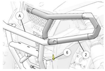
10. Repeat Steps 3-5 for RH bumper 3.11. Install RH bumper 3 to LH bumper 2 using two screws 5.
