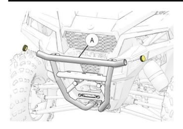
7. Loosely install threaded mount 4 to tapered end of LH bumper 2 using screw 1. Screw should engage only a few threads of threaded mount.
