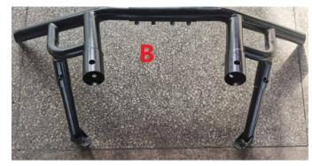
1-3. Assemble Part 4 and Part 5 on Part B with two M8\*50 inner hexagon screws and two M8 locknut to form the rear bar body, as shown in the figure below:
