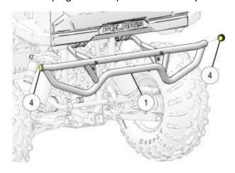
4. Lift bumper 1 as high as possible, then torque all eight screws to specification.
