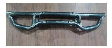
Assemble parts 1, 2, 3 and 4 together with four 8\*50 hexagon socket screws and four M8 locknuts
