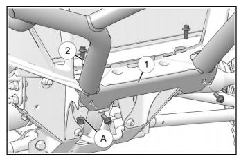
3. Install each arm of bumper 1 with one bolt 2.
