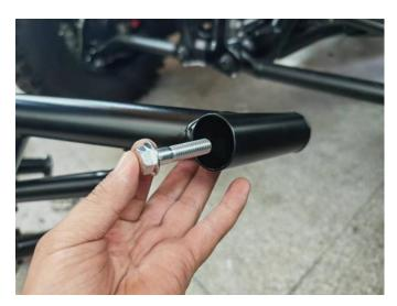
3. Install the lower end of the bumper at the position (shown in the picture) by two M10\*75 nuts with washer and two iron brackets.
