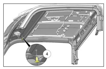
9. Secure rear edge of roof panel to ROPS using four screws (2).
