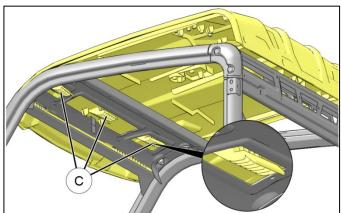
7. Slide roof panel rearward until hooks (C) lock into ROPS visor, then press rear of roof panel down until two tabs (D) snap into B-pillar cross-member.
