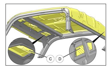
8. Secure front right corner of roof panel to ROPS using screw (4). Repeat for front left corner.
