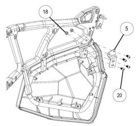
6. Reinstall front and rear upper door panels(C) to upper door frames (A) as shown using six retained screws (B) removed in Step 2. Torque to specification.
