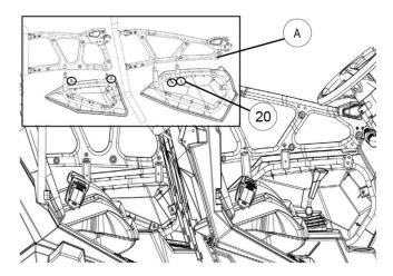
5. Install lower door mount (5) using four screws (20) and two nuts (18) as shown. Torque UPPER two screws to specification.Do not tighten lower two screws at this time.
