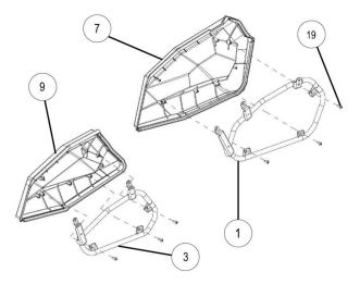
4. Slide lower door subassembly brackets into slots in upper door frame (A), then loosely install two screws (20) per door as shown.
