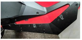
3. Install the door fender with 7 plastic clips as shown in the picture.
