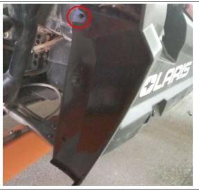
4. Map the three open holes separately onto the holes that come into being in step 1 and step 2,and twist the fillister head hexagon socket screws(black coating)M6X25.(see diagram 1 & diagram 2 on the right)
