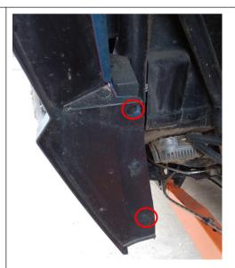
2. Remove the screws on original rear wheel brow(see diagram 1), and mount the L-shaped holder to the inner side of rear wheel brow(see diagram 2), the mounting screws are the original screws you removed just now. Then connect U-shaped nut to the L-shaped holder(see diagram 3). Please choose the hole on the holder as per your vehicle model.
