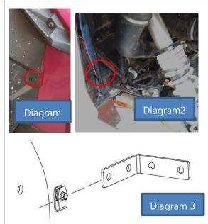
3. Mount the U-shaped nut to the vehicle(see the position in red circle on the right diagram).
