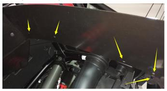
8. There is a part of mud flap above the tail light. Place the mud flap on the plastic parts on the tail light, and drill 2 holes indicated by arrows shown in the following image through the mud flap and plastic parts, then fix them together by 8mm plastic snap fasteners, and complete the installation of rear mud flap.
