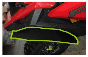
6. There are corresponding holes in the position indicated by the yellow arrow on the rear mud flap and the rear fender. Fix the lower end of the rear mud flap on the rear wheel mud
