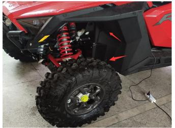
3. Align the two holes indicated by the red arrow on the front fender flare with the mounting holes of the screw removed in step 2. Tighten the screws removed in step 2 on these 2 holes.
