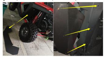
7. Place the rear mud flap under the rear wheel guard panel together, then drill the holes indicated by the arrows shown in the following photo by 8mm drill bit, and fix them together by 8mm plastic snap fasteners.
