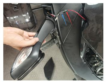
6. Use the white wire to connect from the red arrow position of the fuse in the ACC control box,and connect this white wire to the white wire of the fog lamp cover, to ensure the insulation.
