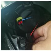
5. Put the other plug of the lamp wiring harness (as red arrow) through the mounting hole of the rearview mirror, and insert it into the plug of the rearview mirror (as blue arrow).
