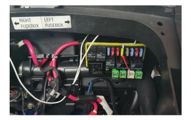
Remark: In order to avoid being cutting off of the wiring ,you can route the wire from ACC control box as the picture.
