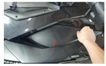
4. Put the wire through the mounting hole of the fog lamp cover; Insert the plug of the lamp wiring harness (as red arrow) into the plug of the original vehicle wiring harness (as blue arrow).
