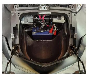
2. Drill a hole at the upper middle of the front bumper by the pistol drill.
