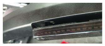
7.Attach one 6mm gasket (circled in red) on the middle pillar. Lock the fender light with clamping rings and self-tapping screws.
