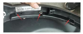
4. Use the perforating template in the packing box ,to drill holes at the right fender flares.
