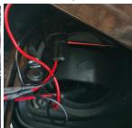
10. Install the splash guards, connect the plugin of fender light to the plugin of patch cord.
