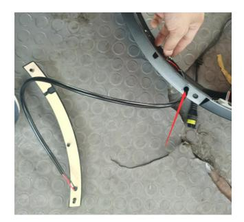
6. Remove the non-stick paper of the double sided adhesive, which is on the back of the light, and stick the light on the fender flares.
