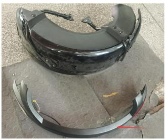
3. Remove the side reflex reflector from the original fender flares, as indicated by the arrows.
