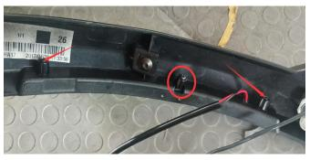
8.Install the fender flares on the splash guard. Sort the wire harness out. Insert the plugins according to the picture.
