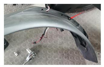
4. Disconnect the plug, take out the original front daytime running light with turn signal light.
