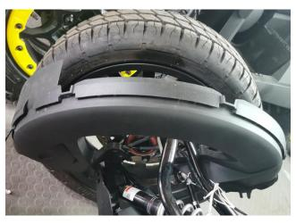
3. Remove the side reflex reflector from the fender flares, and take out the screws as the arrow shows.
