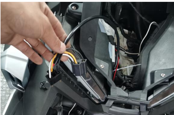
6. Plug the transfer wire plugin of the auxiliary light with the headlight wire plugin.
