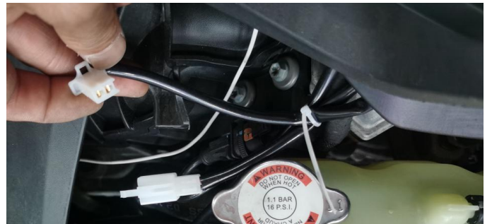
7. Insert the connector of the auxiliary light into the connector of the transfer wire.
