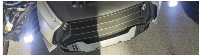
8. Install back the net and cover. Installation finished.
