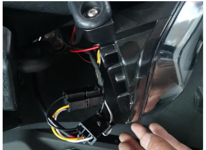
7. Insert the connector of the auxiliary light into the connector of the transfer wire.
